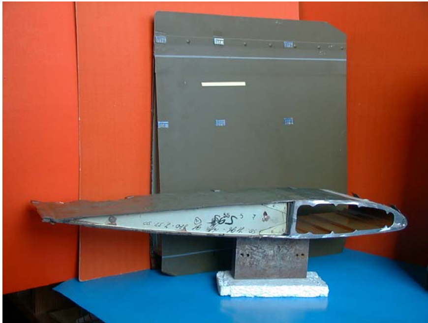
Figure 6: A lying special sample for ultrasonic test.
