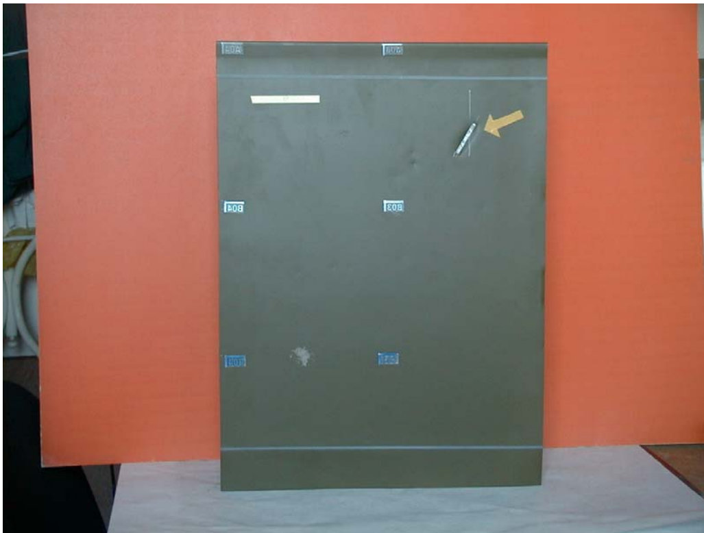
Figure 5: Metal inclusion (at the yellow arrow) in the reference object (original sector).
