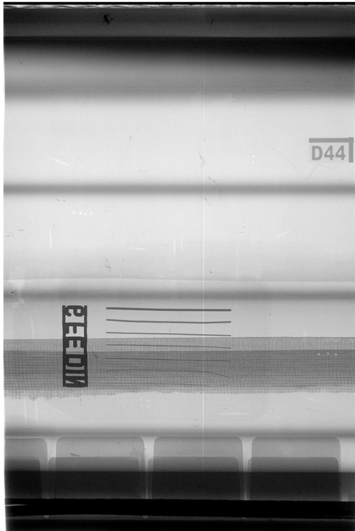
Figure 14: XR picture of the special object (D44 exposed picture field) for UT measurement contains of holes and imitation of cracks with 6FE type picture quality indicator.
